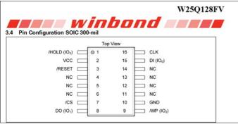
Mémoire flash série : Winbond 25Q128FVFG 3V 128M-BIT SERIAL FLASH MEMORY WITH DUAL AND QUAD SPI
